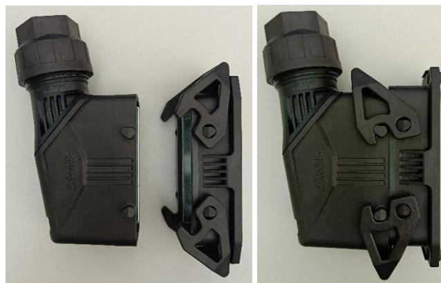
Figure: open (left) and closed (right) female-male connector
