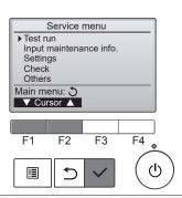
② Select "Test run" with the F1 or F2 button, and press the [ ] button.
