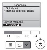
② Select "Remote controller check" from the Diagnosis menu (PAR-4xMAA) or Service menu (PAR-3xMAA), and press the [ ✓ ] button to start the remote controller check and see the check results.
