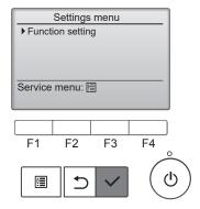
② Set the indoor unit refrigerant addresses and unit numbers with the F1 through F4 buttons, and then press the [ ✓ ] button to confirm the current setting.
