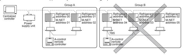
Note: In group B, M-NET address of the outdoor unit whose refrigerant address is "00" is not set to the minimum in the group. As "3" is right for this situation, the setting is wrong. Taking group A as a good sample, set the minimum M-NET address in the group for the outdoor unit whose refrigerant address is "00".
