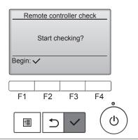
OK: No problems are found with the remote controller. Check other parts for problems.
