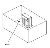
B) Install in a space with a depression height of ≤ 0.125 [m].
