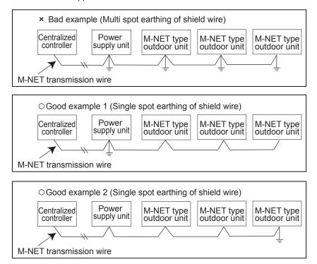
If there are more than 2 earthing spots on the shield wire, noise may enter into the shield wire because the earth wire and shield wire form 1 circuit and the electric potential difference occurs due to the impedance difference among earthing spots. In the case of single spot earthing, noise does not enter into the shield wire because the earth wire and shield wire do not form 1 circuit.
