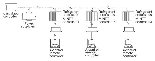
It is acceptable if M-NET wire (non-polar, 2-cores) is arranged in addition to the wiring for A-control.
