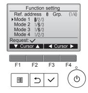
When the settings are completed, press the [ I button to send the setting data from the remote controller to the indoor units.
