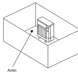
B) Install in a space with a depression height of  $\leq 0.125$  [m].
