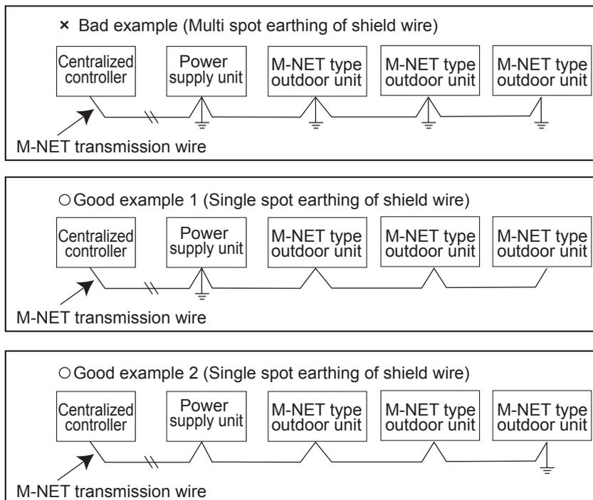
If there are more than 2 earthing spots on the shield wire, noise may enter into the shield wire because the earth wire and shield wire form 1 circuit and the electric potential difference occurs due to the impedance difference among earthing spots. In the case of single spot earthing, noise does not enter into the shield wire because the earth wire and shield wire do not form 1 circuit.
