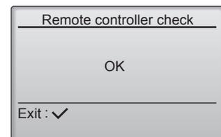
**Check the remote controller display and see if anything is displayed (including lines). Nothing will appear on the remote controller display if the correct voltage (8.5–12 VDC) is not supplied to the remote controller. If this is the case, check the remote controller wiring and indoor units.**
