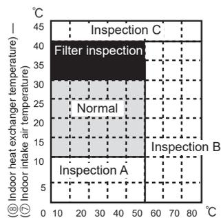
$[(5) \text{ Discharge temperature}] - [(8) \text{ Indoor heat exchanger temperature}]$
