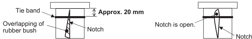
<Back side of the rubber bush (Good example)>
