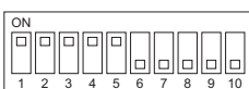
Switches 1 to 5 are ON, and switches 6 to 10 are OFF in the figure on the left.
