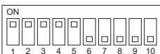
Switches 1 to 5 are ON, and switches 6 to 10 are OFF in the figure on the left.
