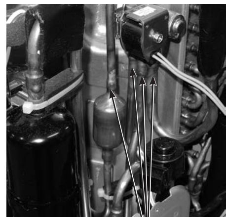
Brazed parts of 4-way valve
