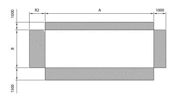
Note: Clearance dimension R2 is from 2500mm to 4000mm depending on model size.
