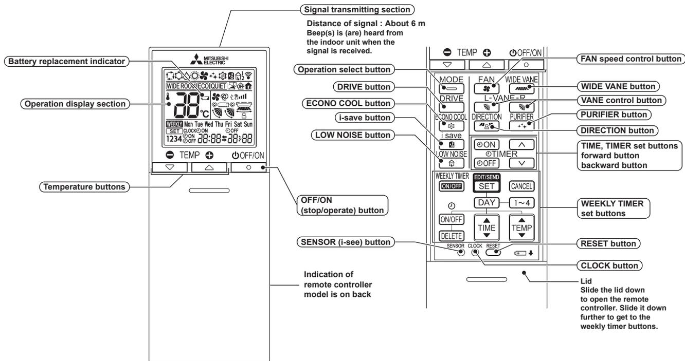
**NOTE:** Last setting will be stored after the unit is turned OFF with the remote controller. Indoor unit receives the signal of the remote controller with beeps.
