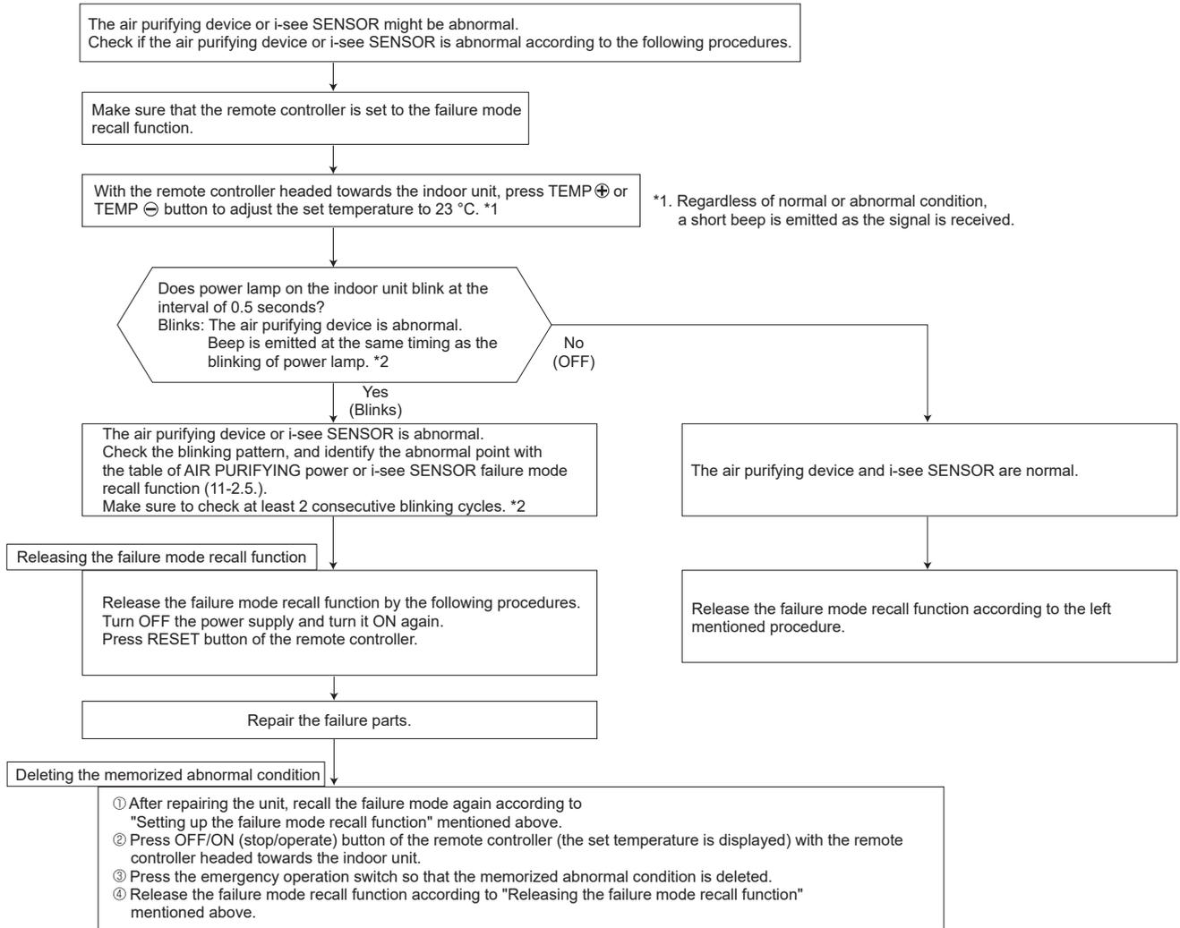
NOTE 1. Make sure to release the failure mode recall function after it is set up, otherwise the unit cannot operate properly.
