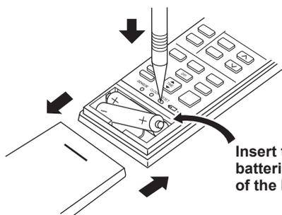
Insert the negative pole of the batteries first. Check if the polarity of the batteries is correct.
