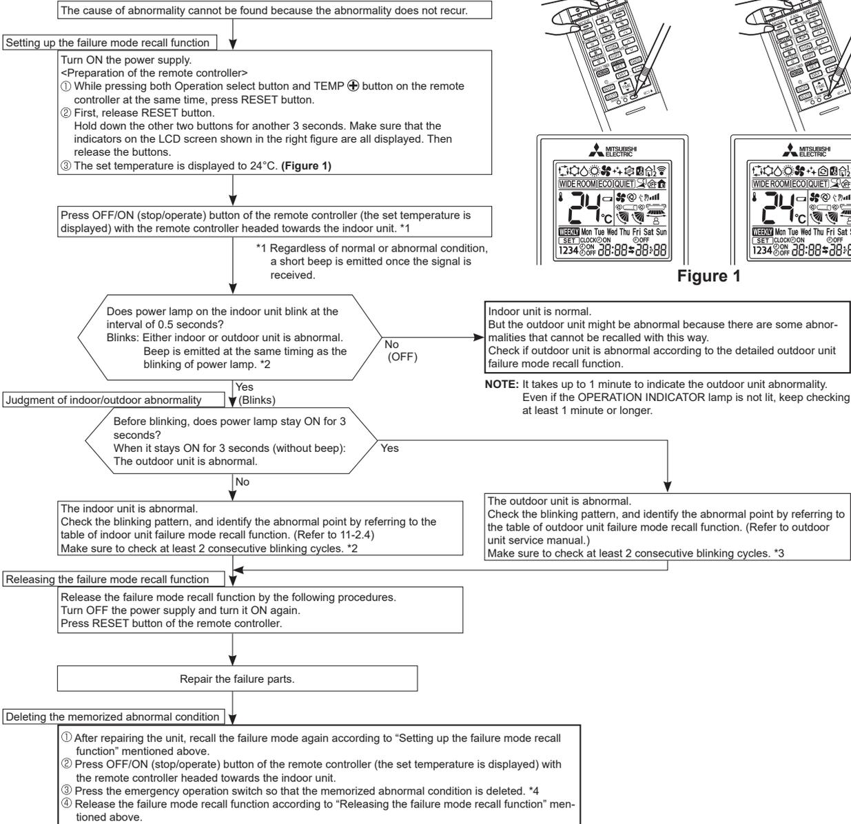
**NOTE:** 1. Make sure to release the failure mode recall function after it is set up, otherwise the unit cannot operate properly.
