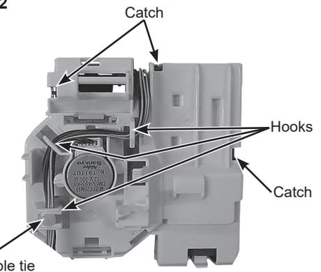
**Back side view of display and i-see sensor assembly**
