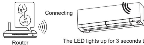
The LED lights up for 3 seconds then blinks twice. A beep sounds as the LED blinks. This series of actions is repeated.
