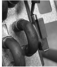
When fixing the indoor coil thermistor to the clip-shape/holder-shape part, the lead wire should point down.
