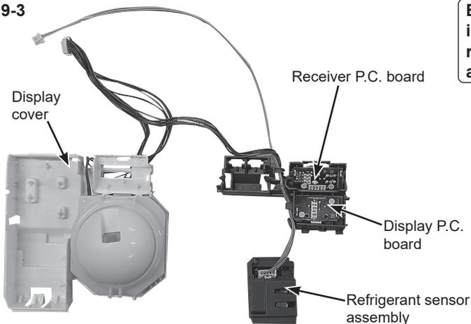
**Exploded view of display cover, display and i-see sensor assembly (display P.C. board, receiver P.C. board), and refrigerant sensor assembly.**
