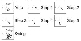
Select "Swing" to move the vanes up and down automatically.
