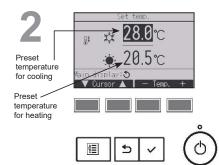
Press the F1 or F2 button to move the cursor to the desired temperature setting (cooling or heating).
