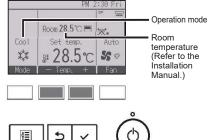
Press the F2 button to decrease the preset temperature, and press the F3 button to increase.
