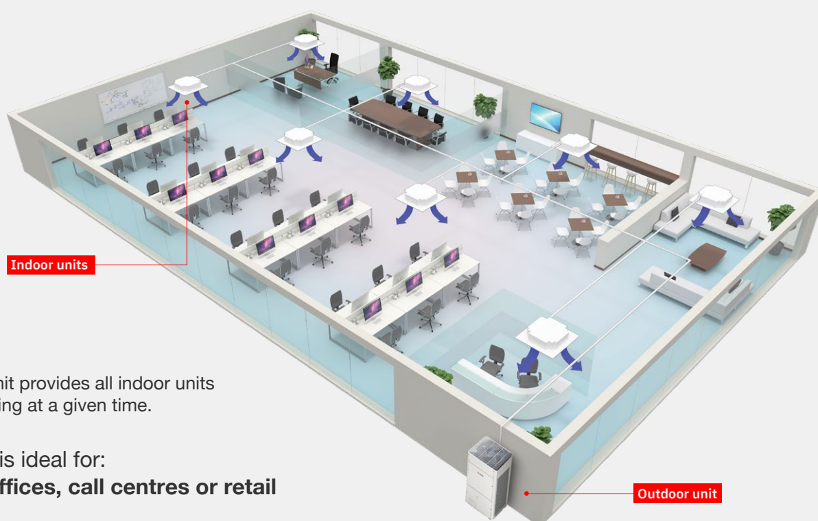
Diagram 1: Mitsubishi Electric Heat Pump VRF System
