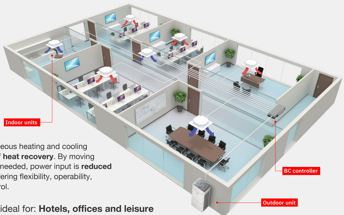
Diagram 2: Mitsubishi Electric's City Multi Heat Recovery VRF System
