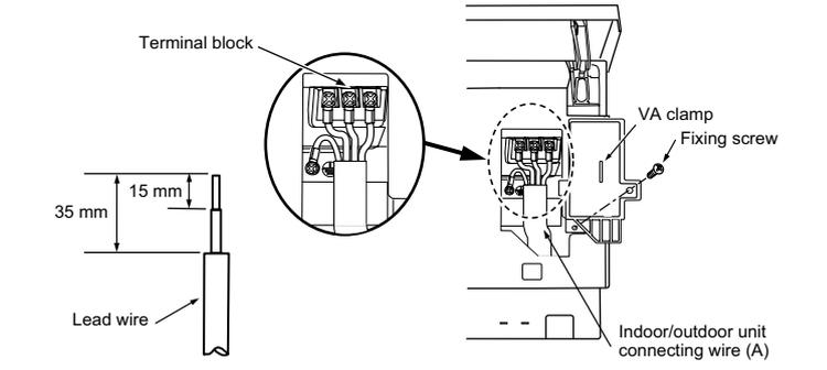
• For future servicing, give extra length to the connecting wires.
