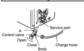
When attaching the control valve to the service port, valve core may deform or loosen if excess pressure is applied. This may cause gas leak.
