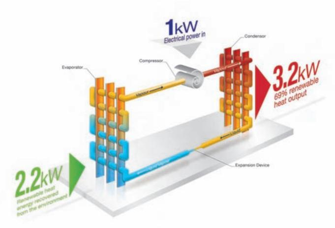
**Ingeniously simple:** Operating in a similar way to a domestic refrigerator in reverse, a heat pump harvests naturally occurring energy, upgrades it and uses it to generate space and/or water heating.
