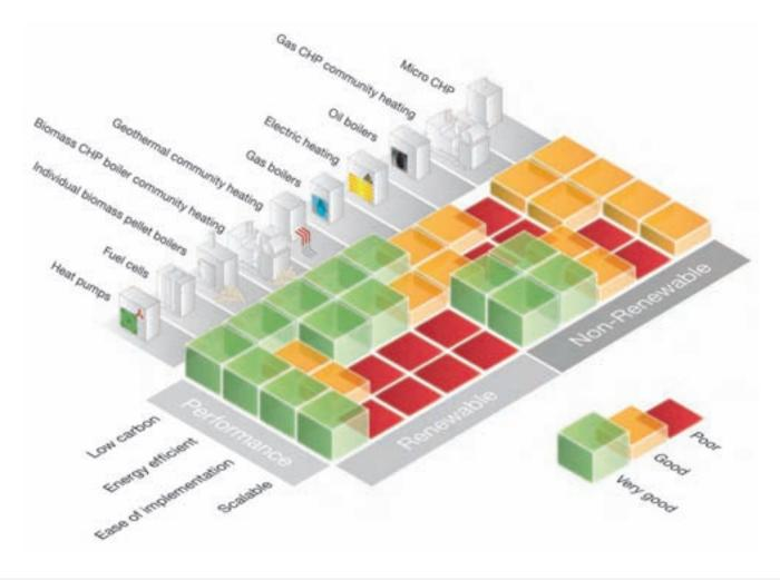
The diagram above is intended to show the Mitsubishi Electric view of how some of the key non-renewable fuelled and renewable heating technologies compare. It does so by highlighting four key areas which are important factors in considering which solutions are effective in terms of both efficiency or carbon reduction and which are capable of rapid mass deployment in order to make a meaningful impact.
