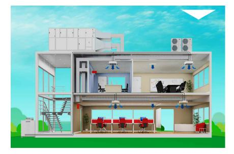
It is also possible to make further energy savings by using free cooling. A damper is incorporated into the AHU which can be adjusted to allow full or partial free cooling using outside air.
