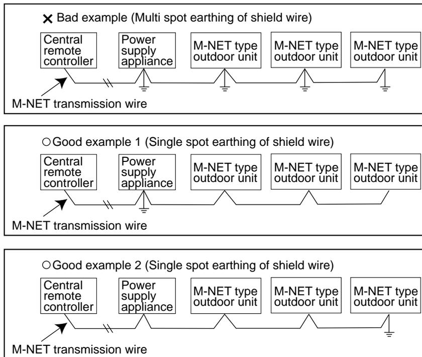
If there are more than 2 earthing spots on the shield wire, noise may enter into the shield wire because the earth wire and shield wire form 1 circuit and the electric potential difference occurs due to the impedance difference among earthing spots. In case of single spot earthing, noise does not enter into the shield wire because the earth wire and shield wire do not form 1 circuit.
