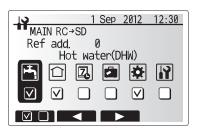
Should settings be changed from default please enter new setting in 'Field Setting' column. This will ease resetting in the future should the system use change or the circuit board need to be replaced.
