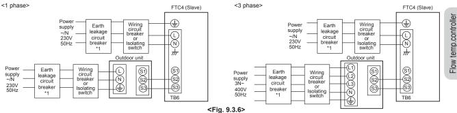
\*1 If the installed earth leakage circuit breaker does not have an over-current protection function, install a breaker with that function along the same power line.
