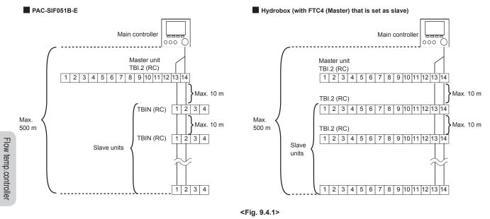
Note: Wiring for main controller cable and daisy chain cable shall be (5 cm or more) apart from power source wiring so that it is not influenced by electrical noise from power source wiring. (Do NOT insert main controller cable and power source wiring in the same conduit.)
