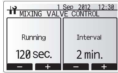
Mixing valve control setting screen
