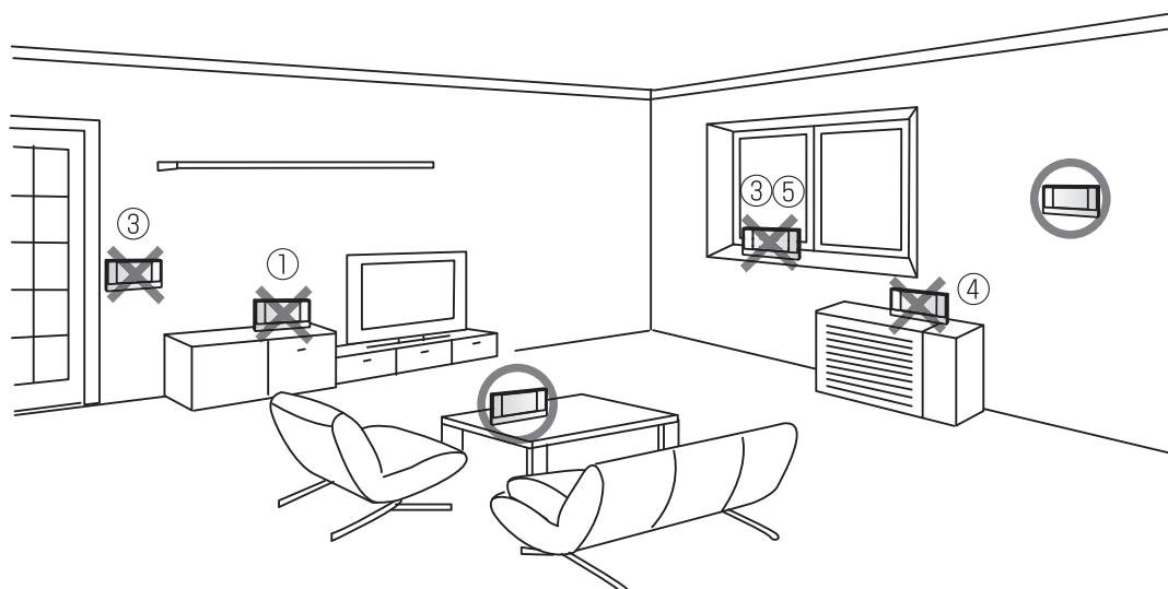
A room sensor is incorporated in each wireless remote controller. If a remote controller is set as room sensor monitoring the room temperature and the wireless remote controller is placed in an improper location, the desired temperature may not be obtained, so select the location to place the wireless remote controller with great care.
