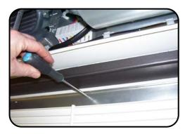
Loosen the row of screws that secure air guide (see picture) and pull air guide up on slots. Do not remove these screws completely.
