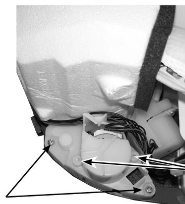
Screws of the horizontal vane motor unit
