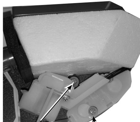
Screw of the vertical vane motor unit
