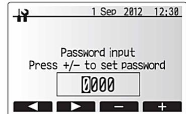
**NOTE:** Manual operation and heat source setting cannot be selected if the system is running. A screen will be displayed asking the installer to stop the system before these modes can be activated. The system automatically stops 2 hours after last operation.
