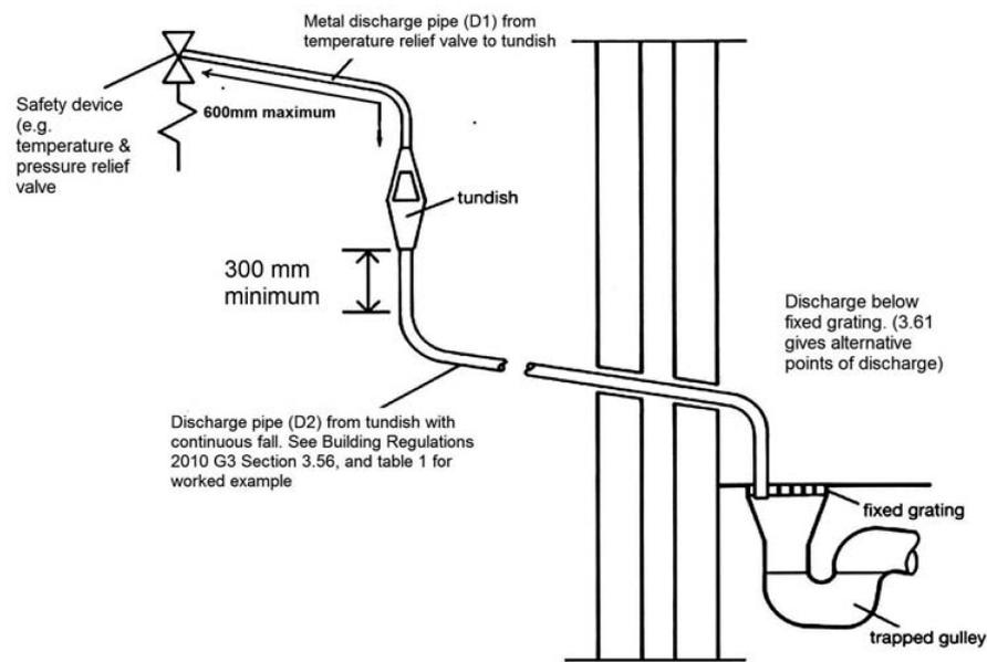
The discharge pipe (D2) from the tundish should:
